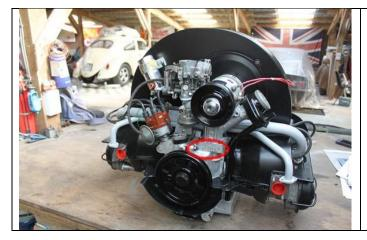
Here is the engine number circled in red, just below the firing order on the generator/alternator pedestal.
