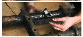
Its okay to do the long anchor screw up tight, but assemble the lock nut/clamp block only finger tight for now. Fit the second suspension arm and its anchor screw. You'll notice that with the two suspension arms and the torsion tube grease seals installed the adjuster 'self-centres' in the beam with a few mm clearance either side.
