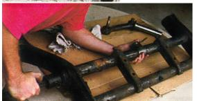
The adjuster needs to be installed dead-centre to the beam. Begin by scribing a line along the beam, through the centre-line of the beams original anchor screw location (highlighted in the picture in red). The width of the adjuster must also be marked on the beam (centre it over the original screw) so a corresponding amount can be cut out. After double checking the marks, a grinder is used to cut the centre from the beam. A few millimetres clearance either side is required, but no more.
