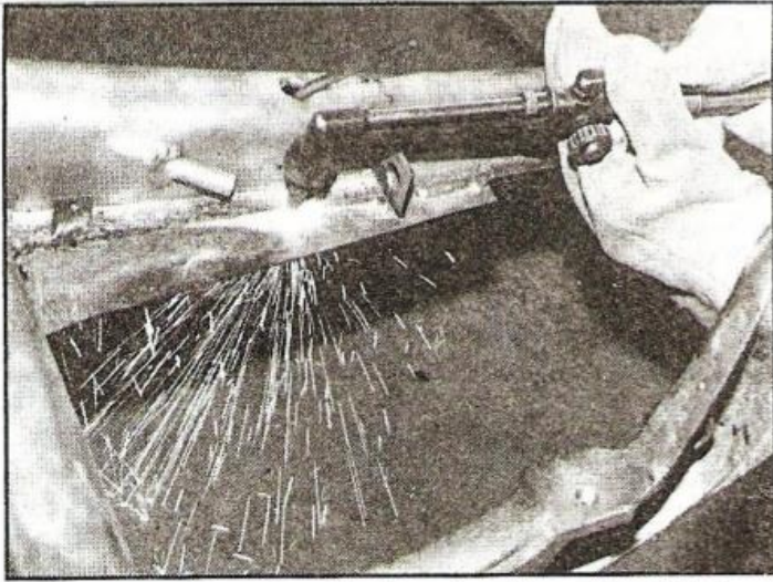
4 A&B-With a cutting torch cut the flange from the rear frame fork, be careful not to cut off the brake hose bracket, and knock it off with a hammer.
